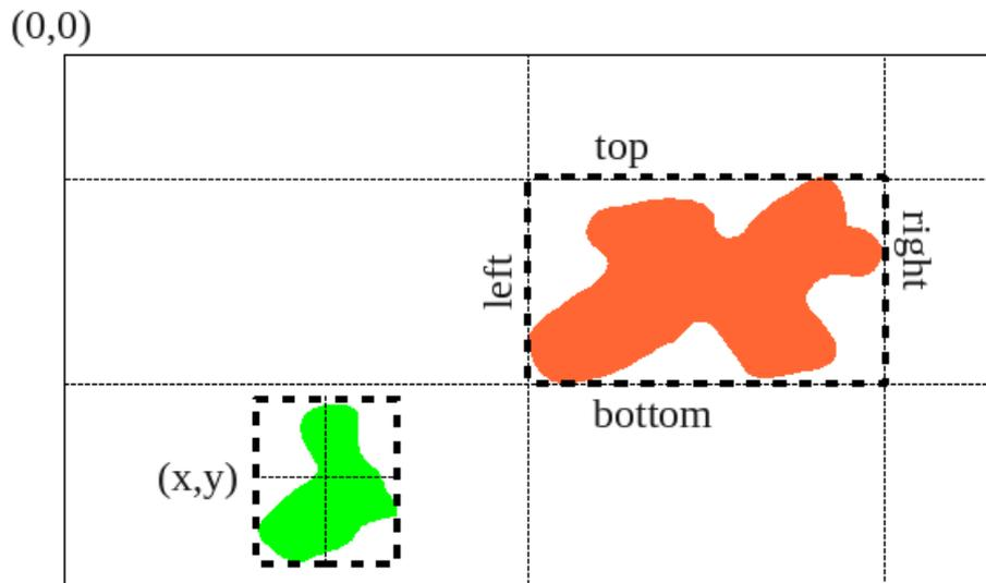
Figure 24: What the fields in `playerc_blobfinder_blob_t` mean. The blob on the left has a geometric centre at  $(x, y)$ , the blob on the right has a bounding box with the top left corner at  $(left, top)$  pixels, and a lower right coordinate at  $(right, bottom)$  pixels. Coordinates are given with reference to the top left corner of the image.
