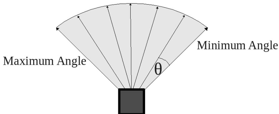
Figure 23: A laser scanner. The minimum angle is the angle of the rightmost laser scan, the maximum angle is the leftmost laser scan.  $\theta$  is the scan resolution of the laser, it is the angle between each laser scan, given in 0.01 degrees.
