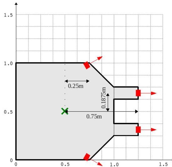
Figure 12: The position of Bigbob's sonars (in red) relative to its origin. The origin is marked with a cross, some of the distances from the origin to the sensors have been marked. The remaining distances can be done by inspection.
