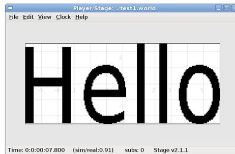
Figure 6: The left image is our "helloworld.png" bitmap, the right image is what Player/Stage interprets that bitmap as. The black areas are walls, the robot can move everywhere else.
