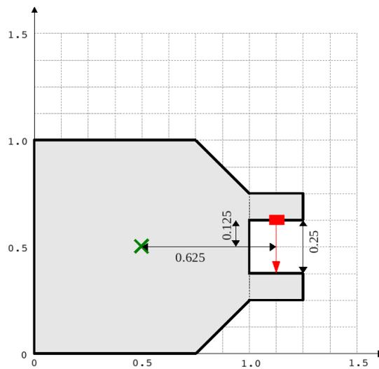
Figure 13: The position of Bigbob's laser (in red) and its distance, in metres, relative to its origin (marked with a cross).
